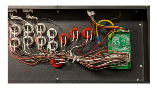
Since the inside of the Hit Box is metal, we want to ensure that the UP5 board does not come into contact with the inside of the Hit Box case.
